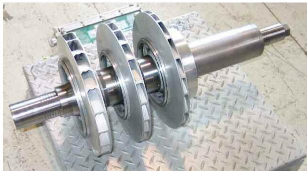
Figure 5. Photograph of Unmodified Compressor Rotor. (Courtesy of Vibration Institute)
