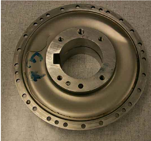
Figure 25. Failure From Angular Misalignment.
