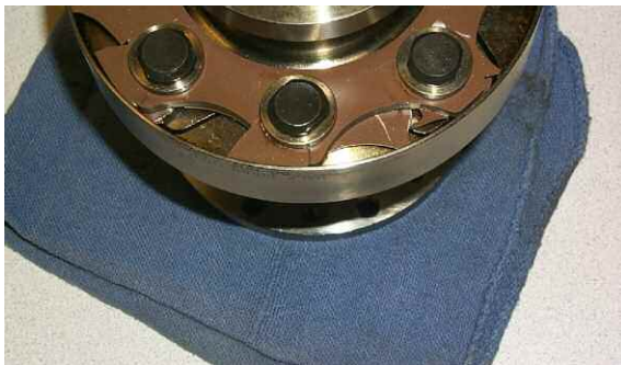
Figure 35. Excessive Angular Misalignment Failure (B).
