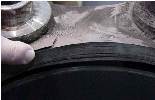
Figure 34. Excessive Angular Misalignment Failure (A).
