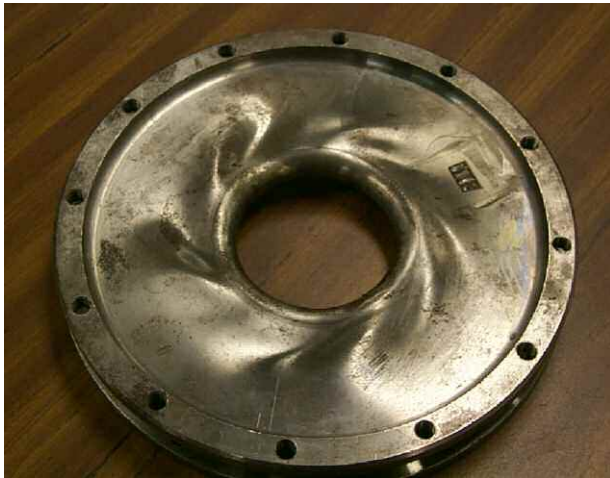
Figure 26. Failure From Torque Overload.
