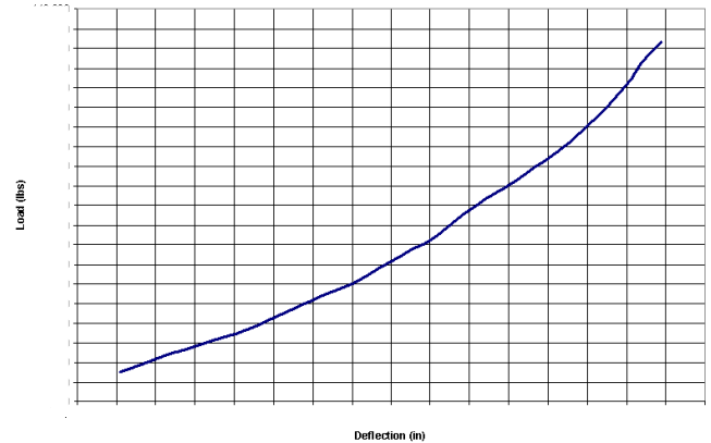
Figure 15. AVM load versus deflection curve supplied by AVM vendor.
