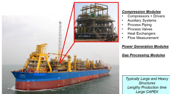
Figure 1. Typical FPSO Arrangement Using Conventional Compression Modules.
