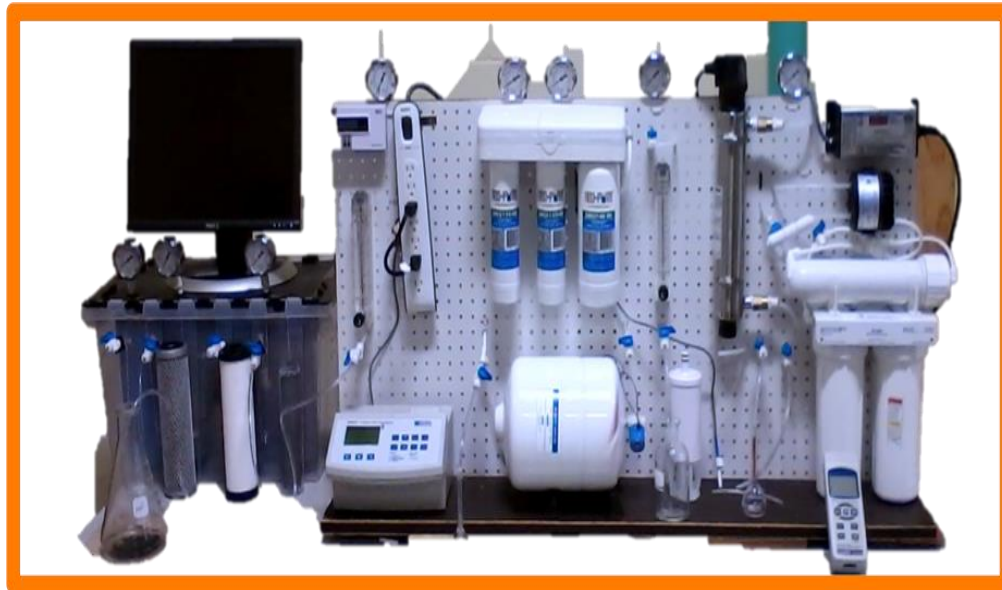
GAC-MI-ME greywater treatment system
