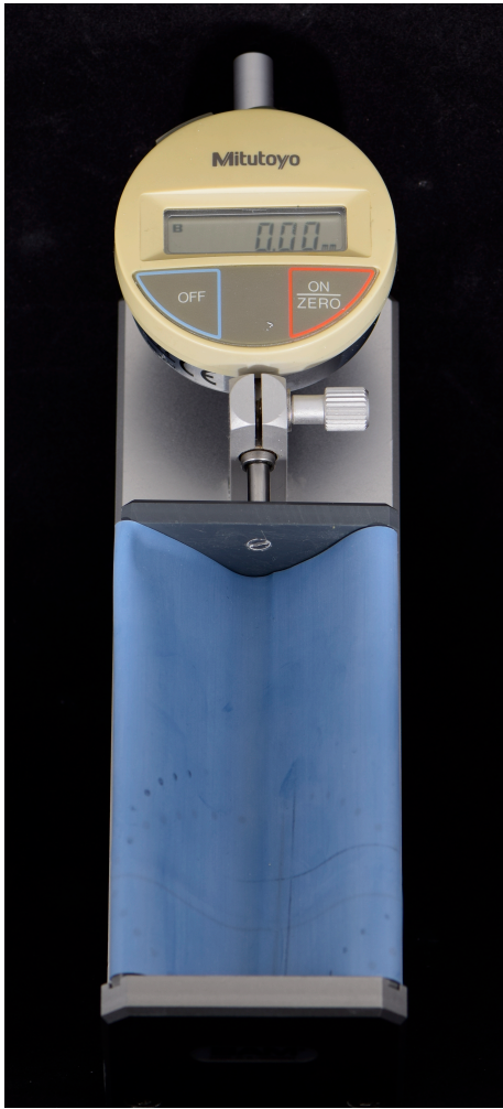
Figure 1. Mitutoyo Digimatic expansion gauge with V shaped trough lined with rubber dam.
