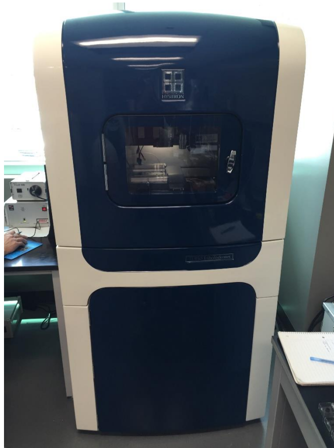
Figure 23 – Hysitron TI-950 Nanoindenter located at the Texas A&M University – Microscopy Characterization Facility.
