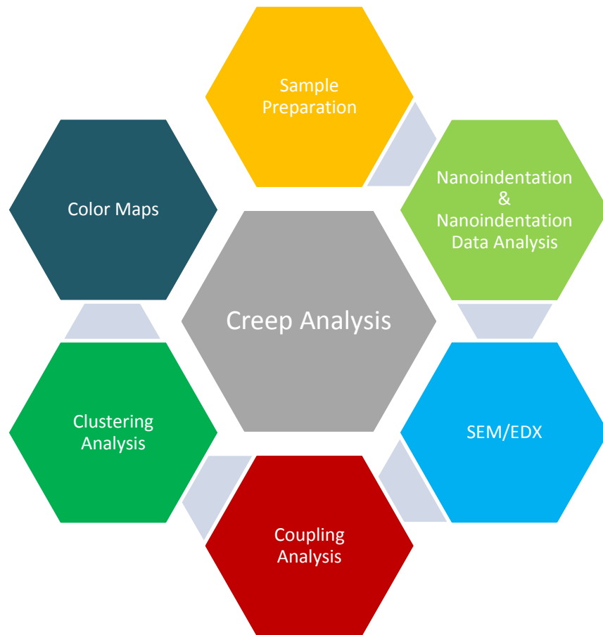
Figure D.1 – Analytical methodology outline to perform creep analysis using nanoindentation and SEM/EDX.
