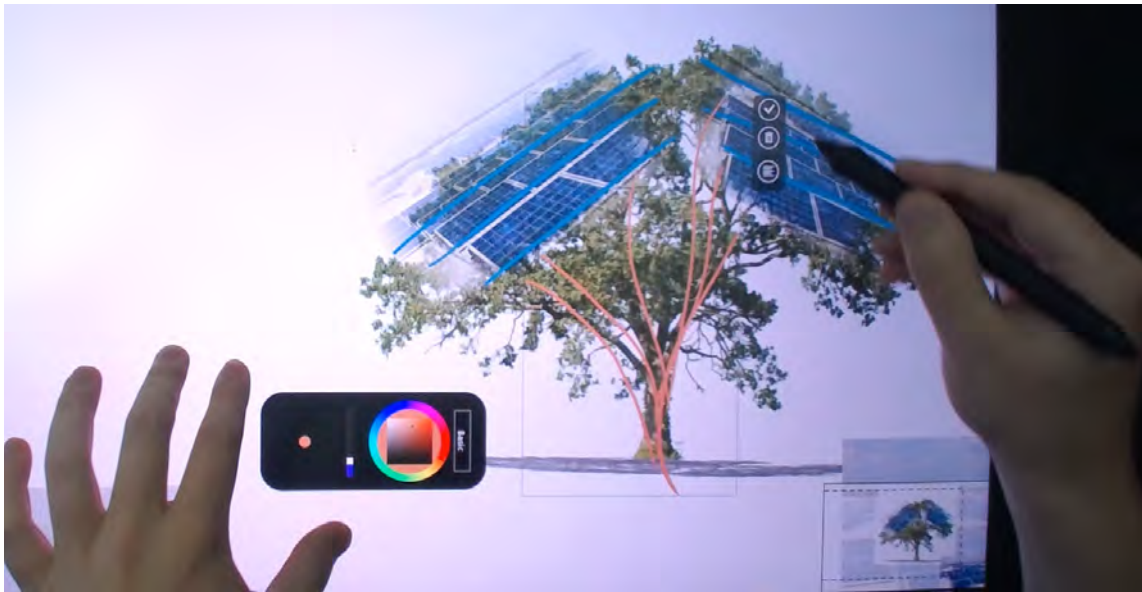
Figure 9: Example of both Ink Menu and Ink Palette activated. In the previous figure, the user changed the ink color to blue. He then draws blue lines on the solar panels to indicate the need for structural pieces to support rows of solar panels. He leaves the Ink Palette activated during this process. After drawing the blue lines, he use the Ink Palette to change the ink color to orange. Then, he traces orange lines over the branches and trunk of the tree to represent conductive tree-like structures for holding up the solar panels and drawing energy from them. The Ink Menu appears after he finishes sketching these lines. The pen in the right hand moves to press the check mark button to add the orange ink strokes to the diagram.
