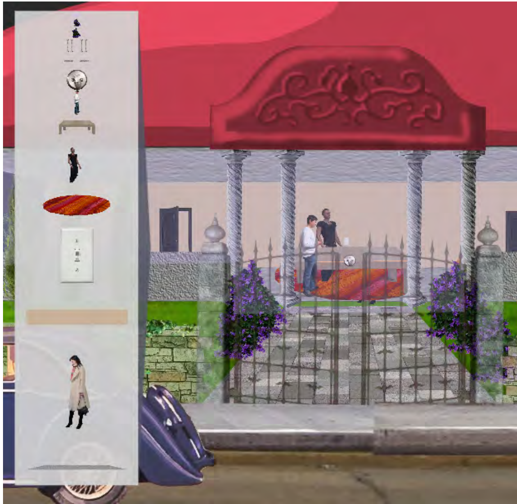
Figure 32: Example of fisheye scene index in LayerFish. The focus of the fisheye is on the correspondent of the woman in a coat. Correspondents get smaller in size further from the focus.
