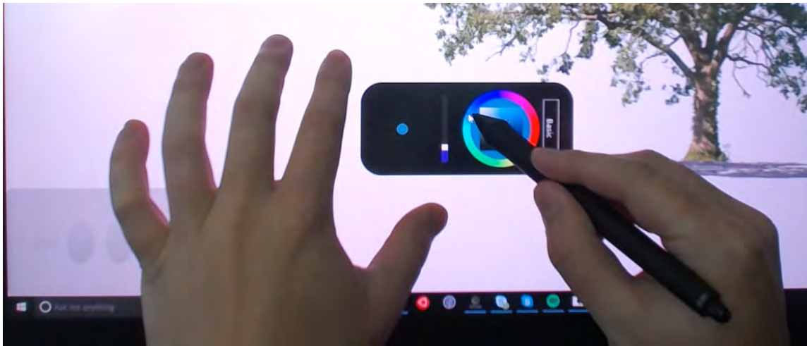
Figure 8: Example of Ink Palette. The left hand performs a right-angle gesture to activate Ink Palette. The right hand, with the pen, adjusts the hue of the ink to a shade of blue.
