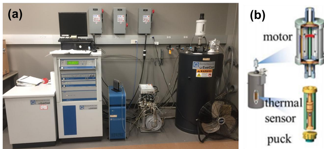
Figure 2.8 (a) The Quantum Design PPMS equipment in the laboratory. (b) The sample motor drive and detection coil set for VSM option.
