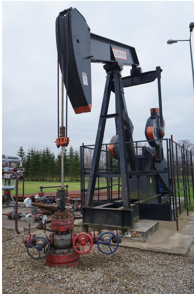
Figure 2 : A sucker rod pumping system.
