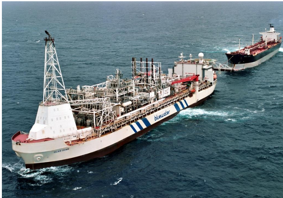
Figure 2: Typical FPSO while transferring oil to a shuttle tanker adapted from [4]
