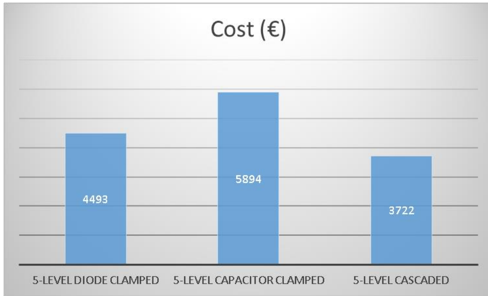
Figure 31: Cost comparison between multilevel inverter topologies
