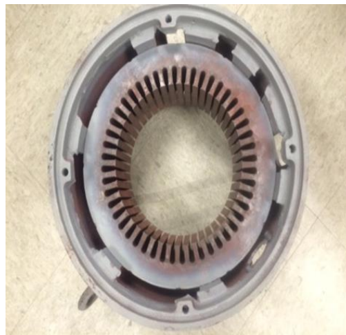
Figure 77: Stator of the synchronous generator with no windings
