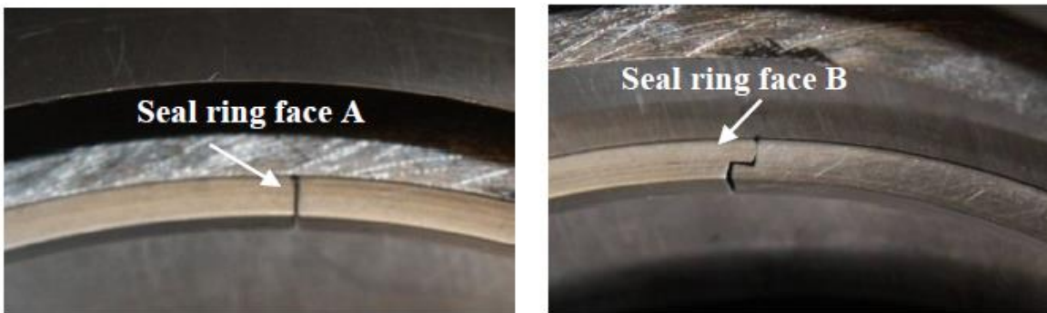
Fig. 26. Proper installation of piston ring in bearing cartridge: face A towards ambient [14].
