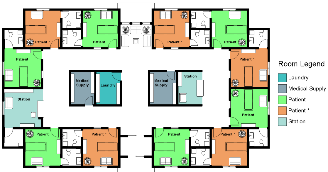
Figure 3-28: The layout of a ward which includes 11 single patient rooms, two medical supply rooms and a laundry room.
