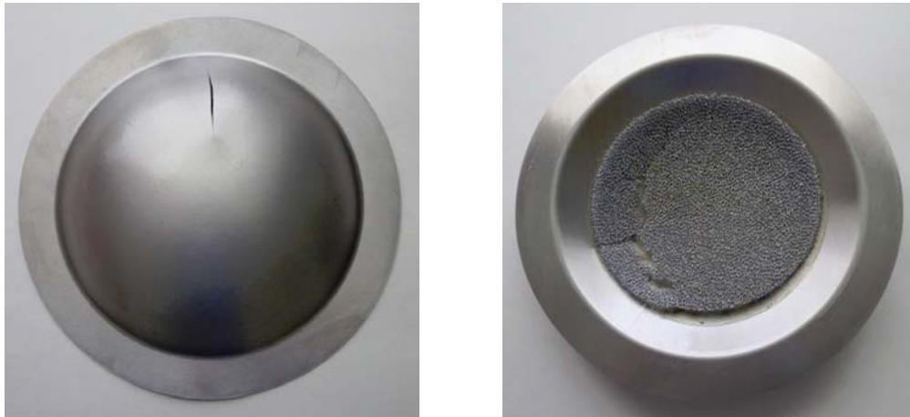
Figure 68 The mixed failure mode in the two-layered panel.
