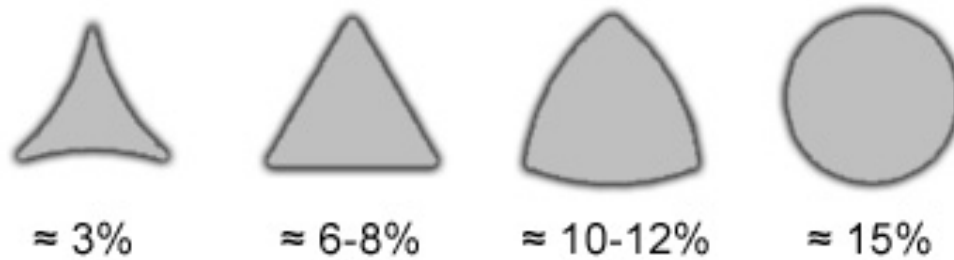
Figure 9 Ligament cross-section profile of Duocel open-cell foam at various relative density [6].
