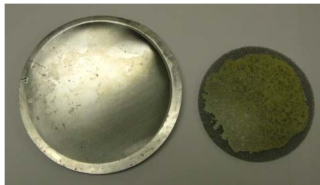
Figure 66 Delamination between the top face sheet and the foam blank.
