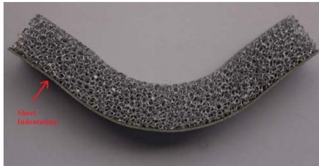
Figure 27 Sheet indentation at 7.69%, 15 mm foam thickness, radius 30 mm test.
