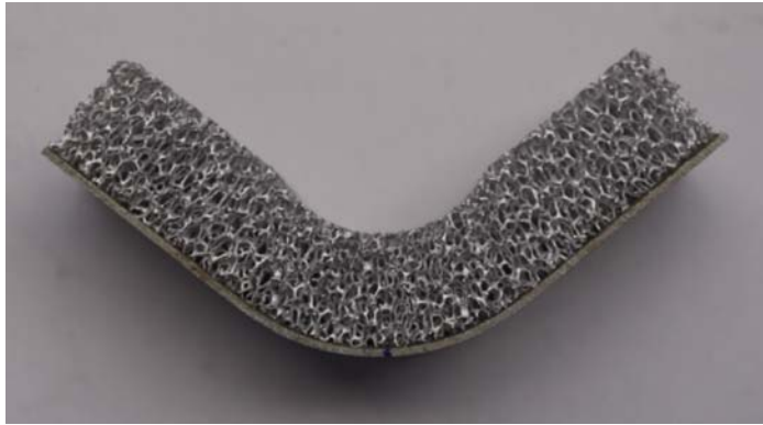
Figure 25 Foam indentation at 4.85%, thickness 12.8 mm foam, radius 10 mm test.
