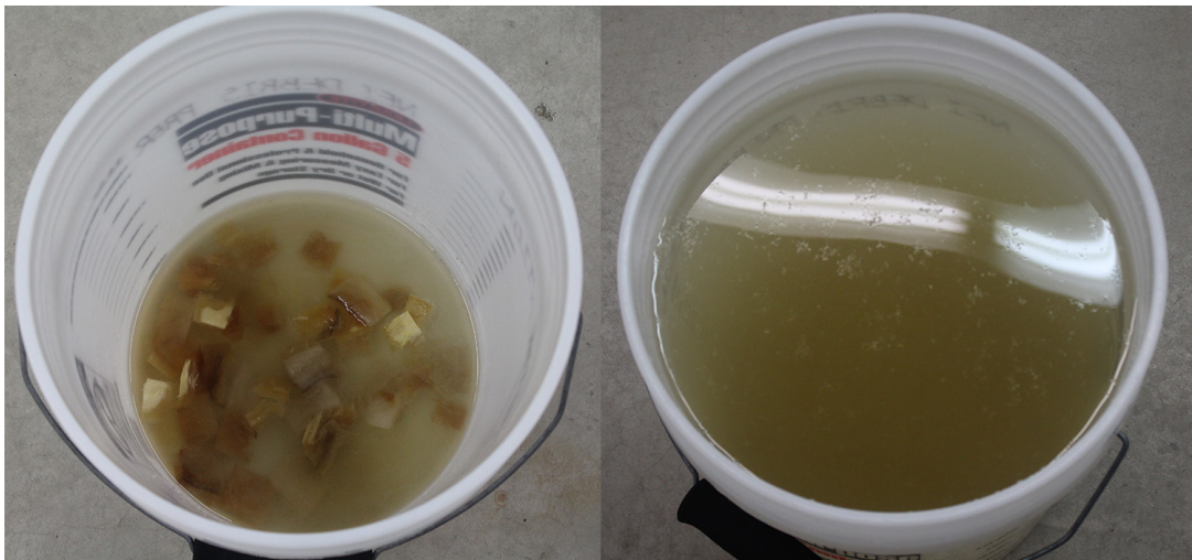
Figure 5.6: Nukon bucket filling process (the 0.5 gallon mark is seen left and the 5 gallon mark is seen right).
