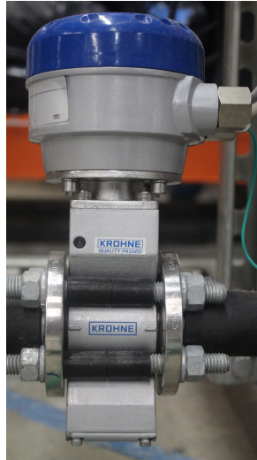
Figure 4.9: Krohne Optiflex 1000 F electromagnetic flowmeter.
