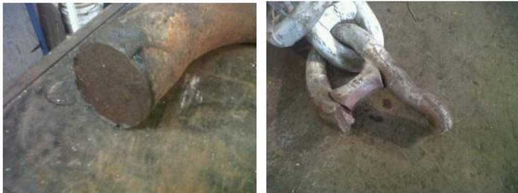
Figure 4.1 The Anchor Chain Failure of Gryphon (Finucane, 2012)
