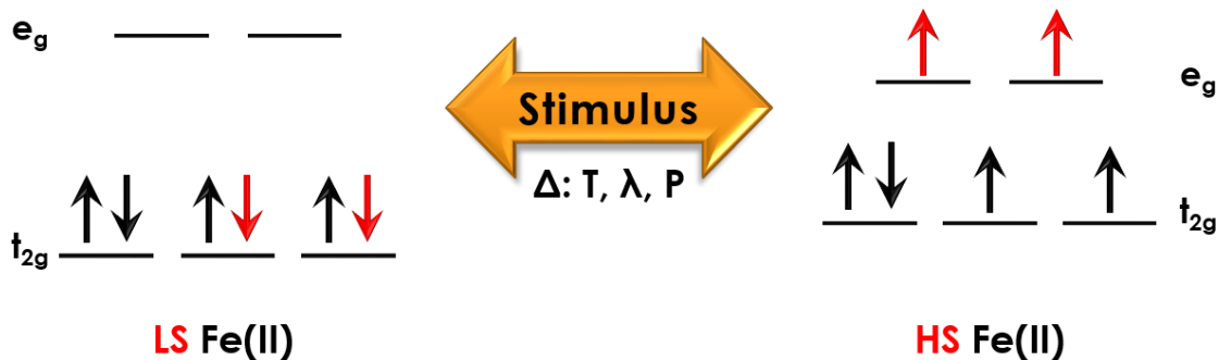
Figure 1-6. Depiction of the electron configuration for the LS and HS states of an Fe II metal center in an octahedral coordination environment that undergoes SCO upon an external stimulus.
