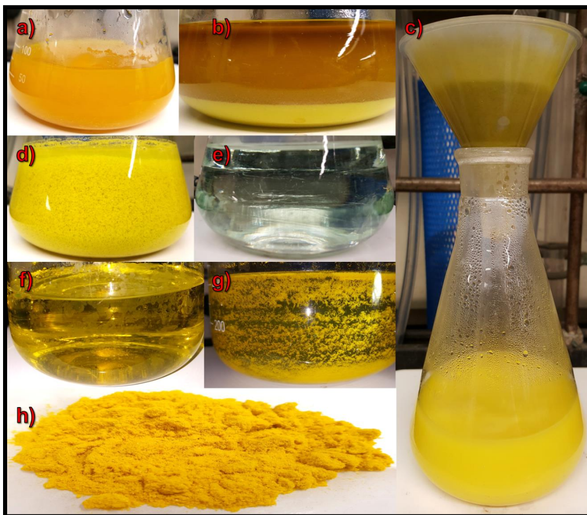
Figure 2-3a-h. Typical colors expected as the synthesis of 1 progresses.
