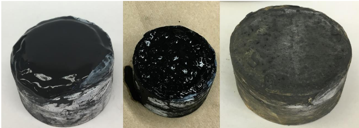
Fig. 12 - Left: Filter cake after static filtration at 300 psi and 250°F; middle: filter cake after soaking with 7.5 wt% HCl at 300 psi and 250°F; right: filter cake after drying at 212°F for three hours.
