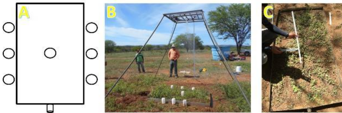
Figure II.3: (A) Representation of the 2-m x 1-m plots with the seven evenly distributed rain gauges. (B) A rainfall simulation in progress on one of the plots in the AP site. (C) A plot in the YF site, where a researcher is measuring the slope and estimating cover.
