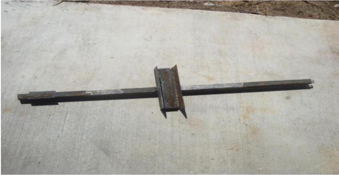
Figure 8: TAMU balanced bond wrench by Chaudhari (2010)
