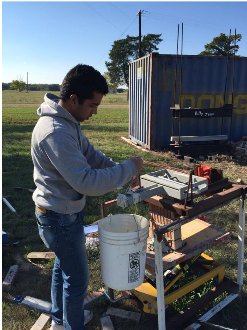
Figure 24: The experiment setup with the bond wrench and prism ready for loading through addition of loads in the bucket.
