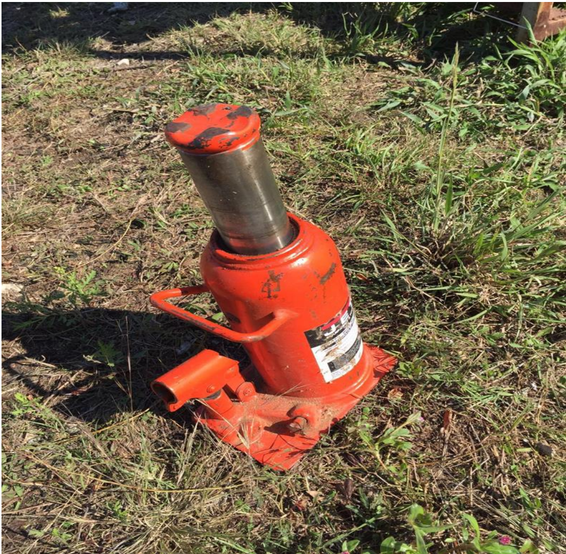
Figure 22: Hydraulic jacks used to lift the specimen in the experiment
