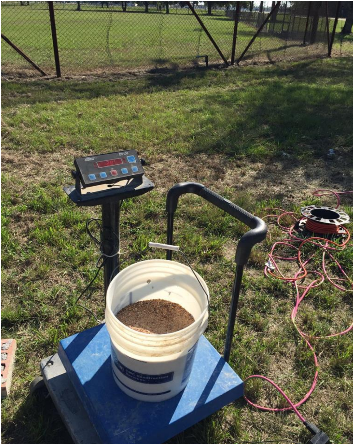
Figure 23: Measurement of the weight needed to break a bond
