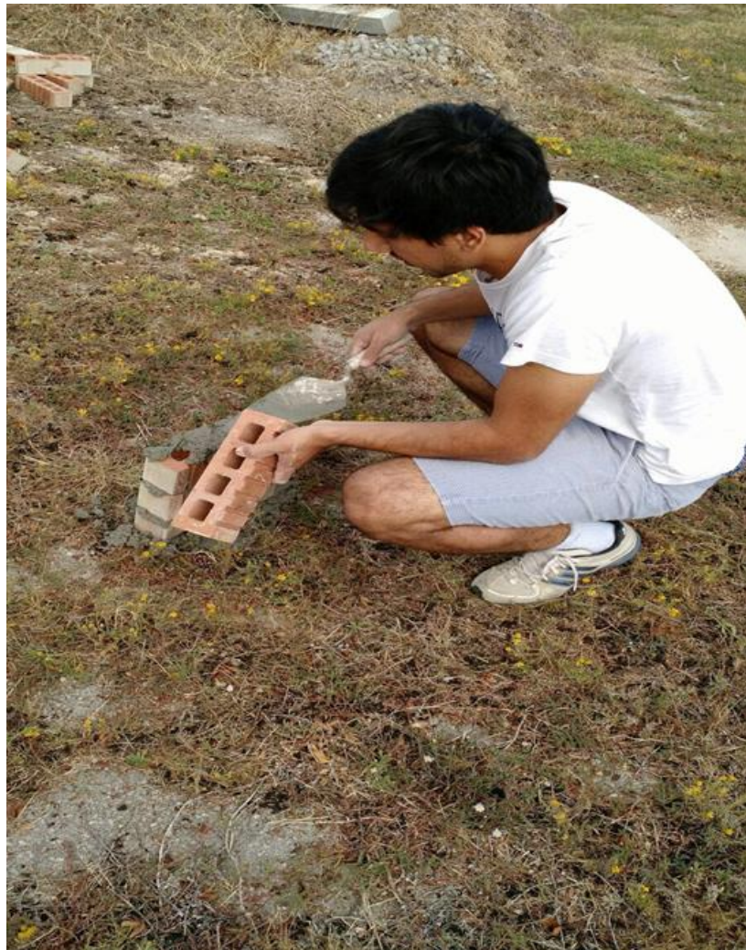
Figure 16: Process of making brick prism
