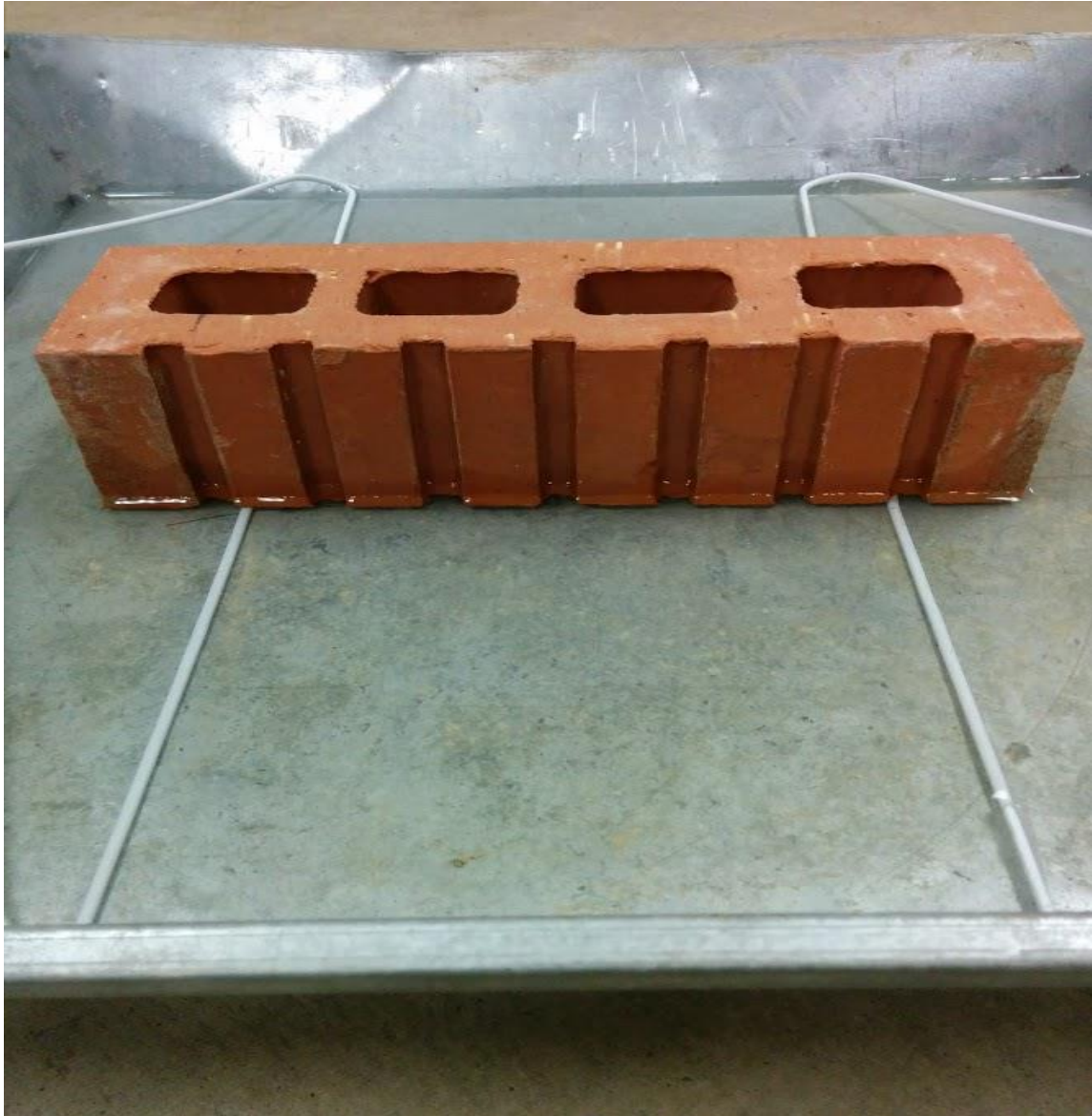
Figure 27: Absorption test on sample brick
