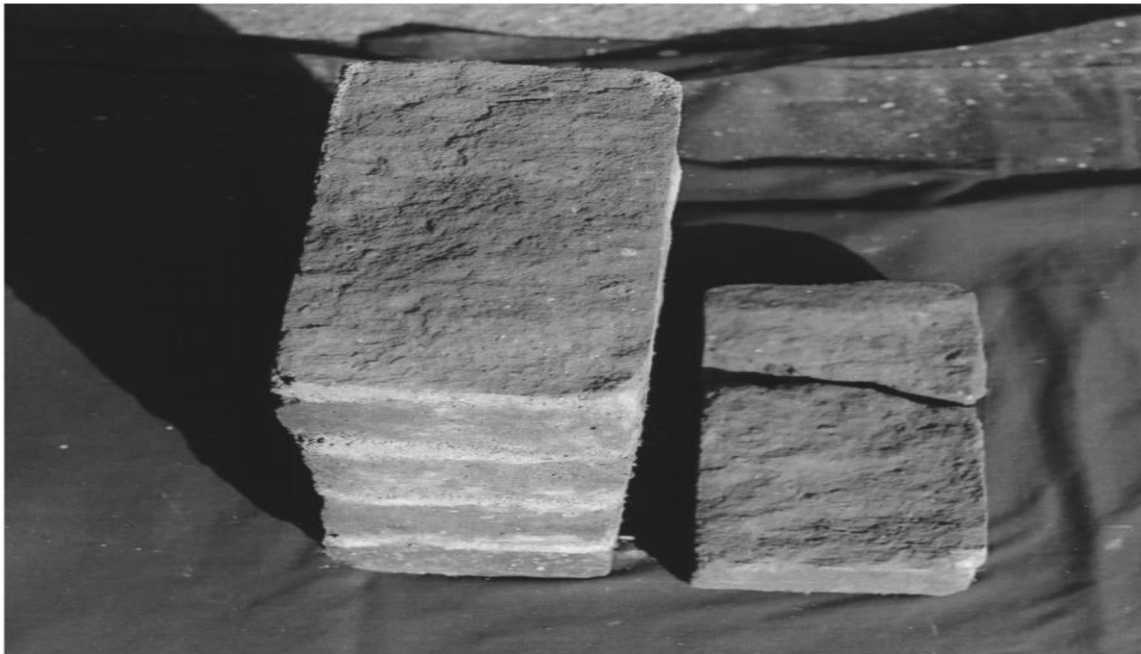
Figure 11: Bond failure when the mortar is still intact (Sarangapani et al., 2005)
