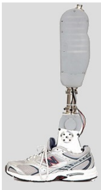
Figure 1.3: The Vanderbilt prosthesis is a powered transfemoral device, developed at the Center of Intelligent Mechatronics in Vanderbilt University.
