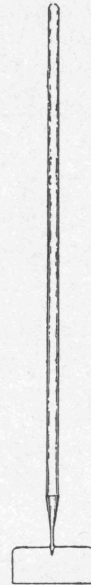
Silage cutter to get silage out that has been put in the trench uncut.
