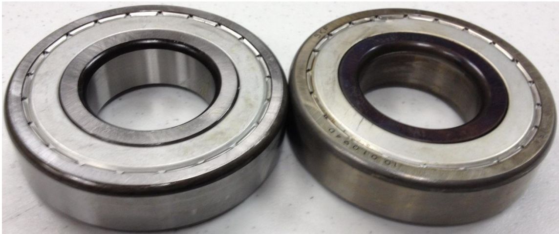
Fig.72 Galling between bearing and shaft under shaft current injection
