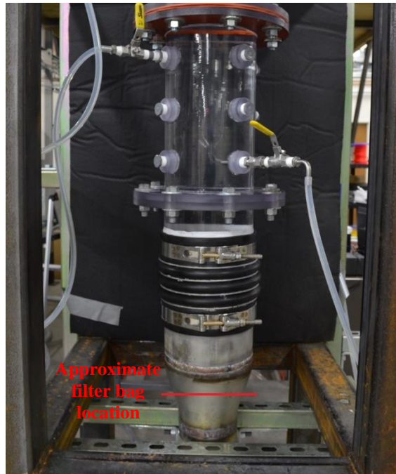
Figure 50. Approximate location of the filter bag installation
