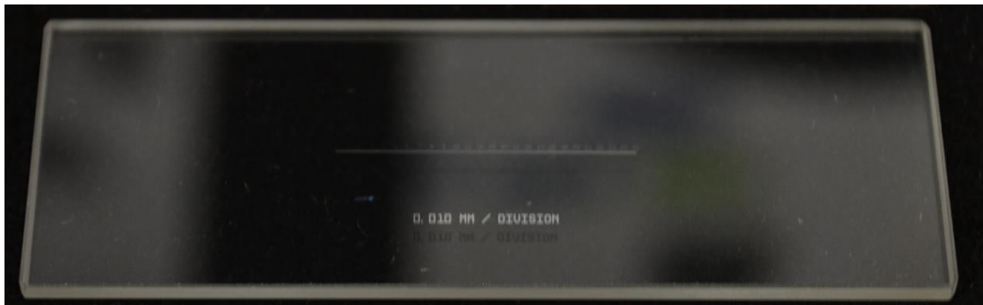
Figure 30. Klarmann Rulings, Inc. KR-838 stage micrometer
