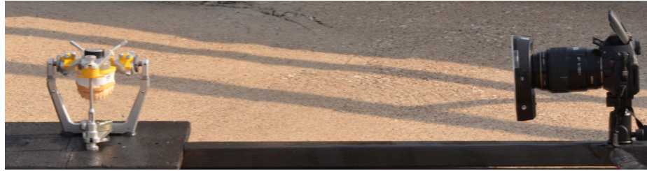
Figure 3: Photo jig with articulator in a stationary reproducible position and Dolica tripod ball head attached 3 feet away.
