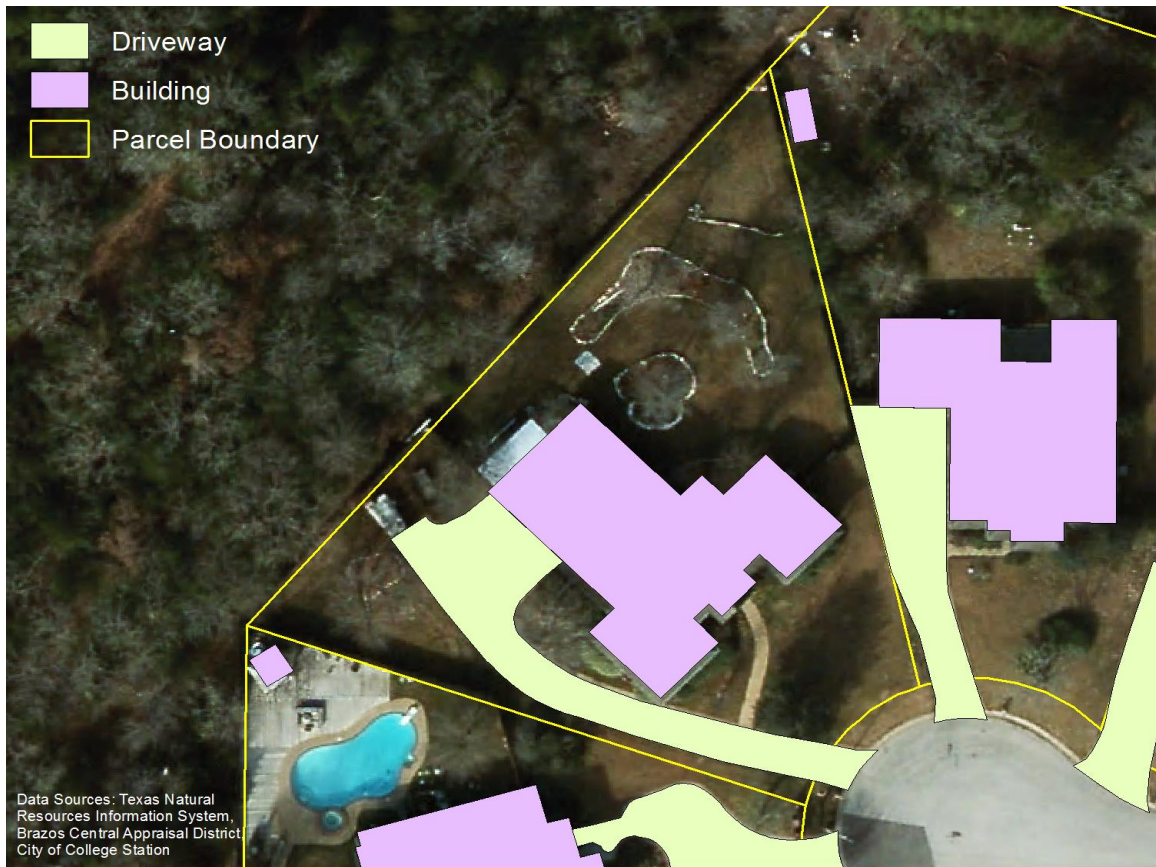
Figure 5. Close-up of GIS layers indicating delineations of lot boundaries, structures, and driveways.
