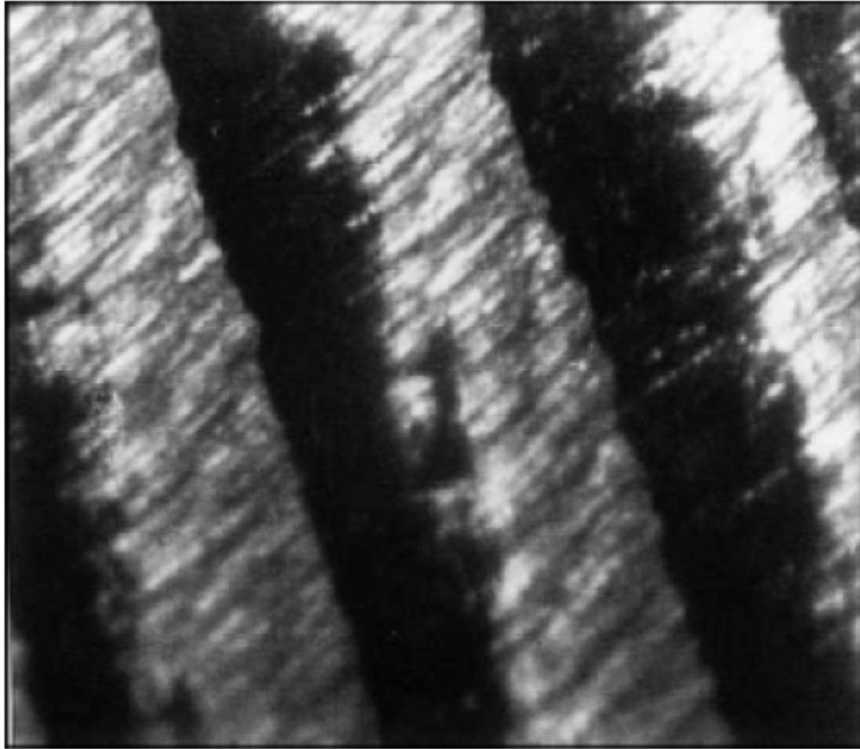
Figure 3.1: Chatter visible as dark bands on the surface of a metal [5]. This figure is reprinted with permission from "Sources of Nonlinearities, Chatter Generation and Suppression in Metal Cutting" by Marian Wiercigroch and Erhan Budak, April 2001, Philosophical Transactions of the Royal Society A: Mathematical, Physical and Engineering Sciences, vol. 359, no. 1781, pp. 663-693, © 2014 The Royal Society.
