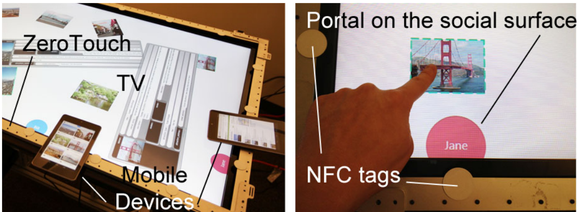
Figure 2.6: Cross-surface interactive system with 55" flat-screen display, ZeroTouch sensor, NFC tags, and mobile devices.
