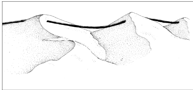
(b) A free cable span between sand waves
