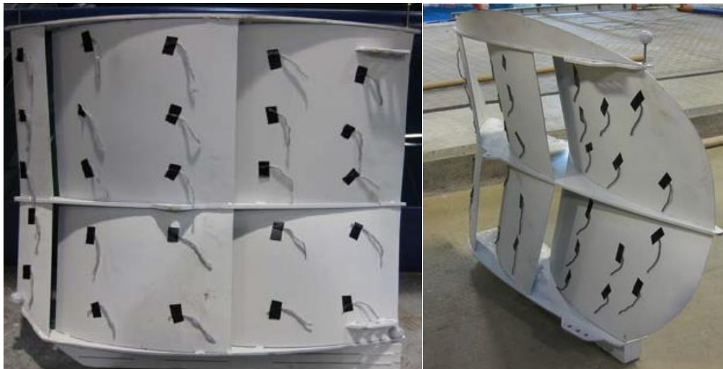
Fig. 1.6 Front and side view of a scaled trawling board model (Teigen et al., 2009)
