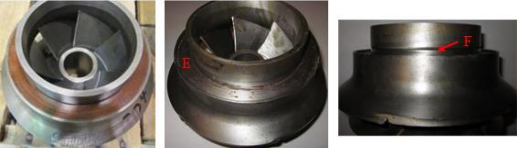
Figure 41. Untested (left) and WAS tested (middle and right) second stage impeller inlet. The middle image shows the worn away eye thrust bearing (E). The right image shows the front ring seal groove (F).
