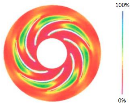
Figure 11. Local GVF field in an impeller supplied by a 17% GVF stream [17]
