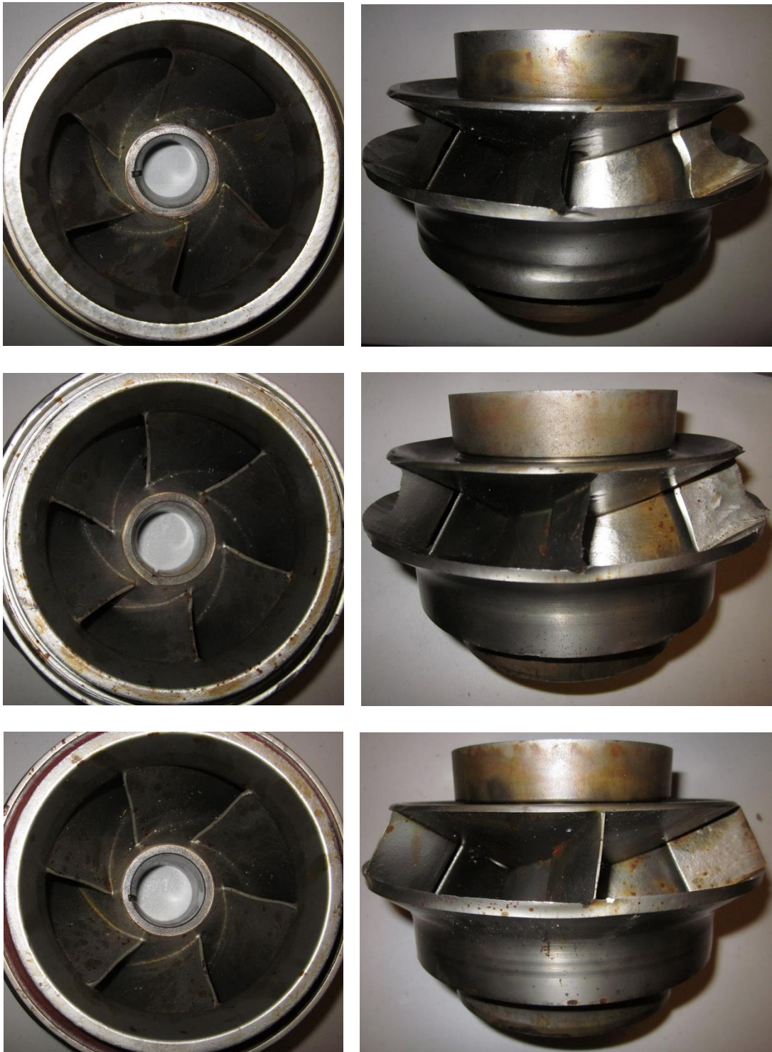
Figure 45. WAS tested first stage (top), second stage (middle), and third stage (bottom) impeller. Inlet views are displayed on left and outlet views are displayed on right.
