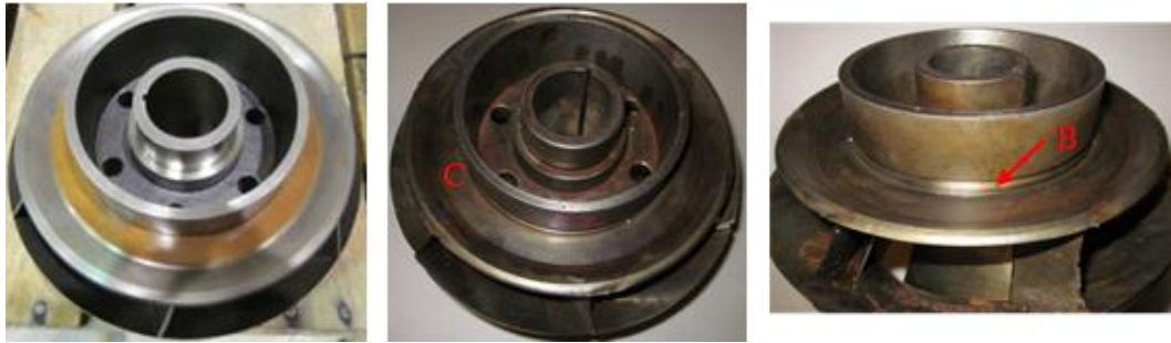
Figure 40. Untested (left) and WAS tested (middle and right) second stage impeller outlet. The right image shows the back ring seal groove (B). The middle image shows the worn away up-thrust bearing (C).
