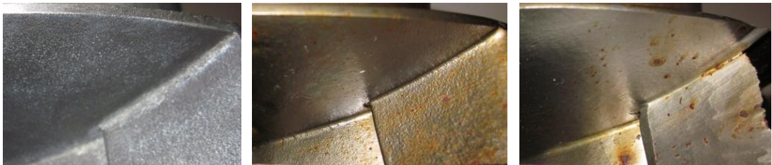
Figure 31. Untested (left), WS tested (middle), and WAS tested (right) second stage hub sidewall
