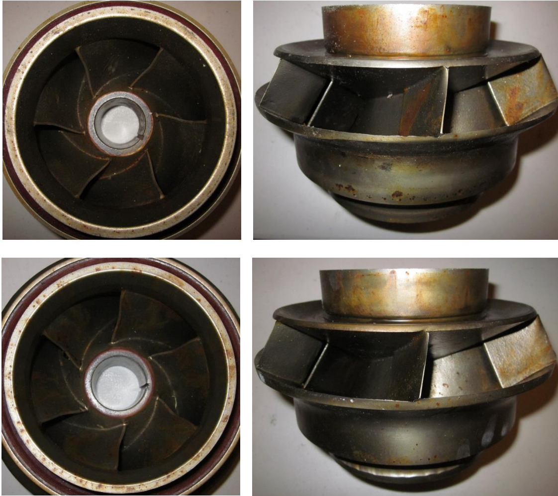
Figure 44. WS tested first stage (top) and second stage (bottom) impeller. Inlet views are displayed on left and outlet views are displayed on right.
