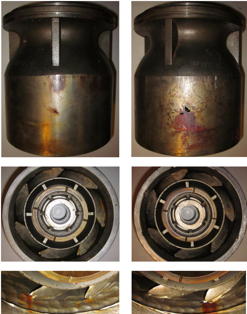
Figure 46. WS tested first stage (left) and second stage (right) diffuser. Side views are displayed at top, inlet views are displayed in middle and a close-up inlet view of two diffuser vanes is displayed on bottom.
