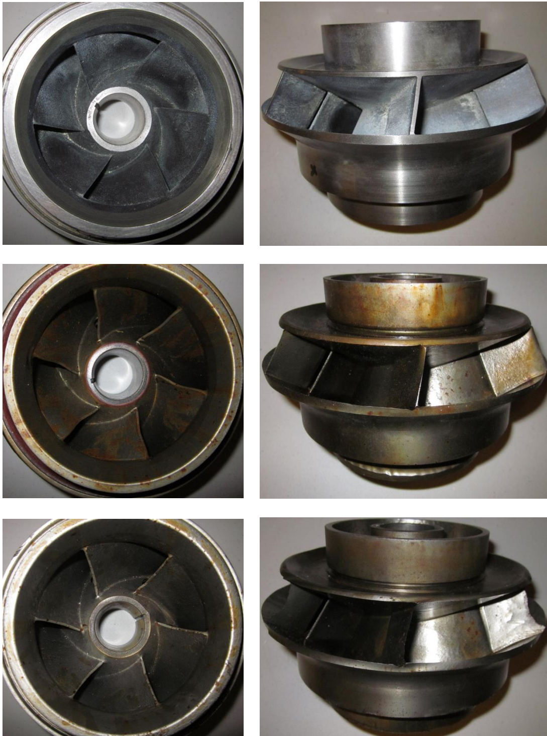
Figure 32. Untested (top), WS tested (middle), and WAS tested (bottom) second stage impeller. Inlet views are displayed on left and outlet views are displayed on right.
