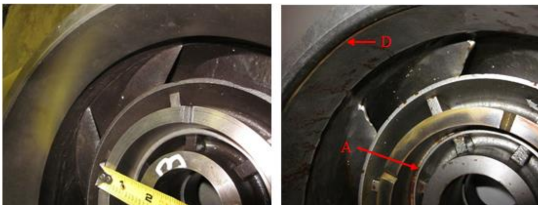
Figure 39. Untested (left) and WAS tested (right) second stage diffuser inlet. The right image shows the back ring seal mate end groove (A) and diffuser lip groove (D).
