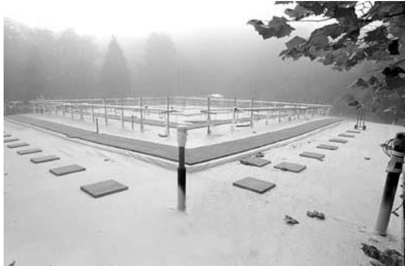
Figure 2.4 Frozen soil barrier system at Oak Ridge National Laboratory (Johnson et al., 2000)
