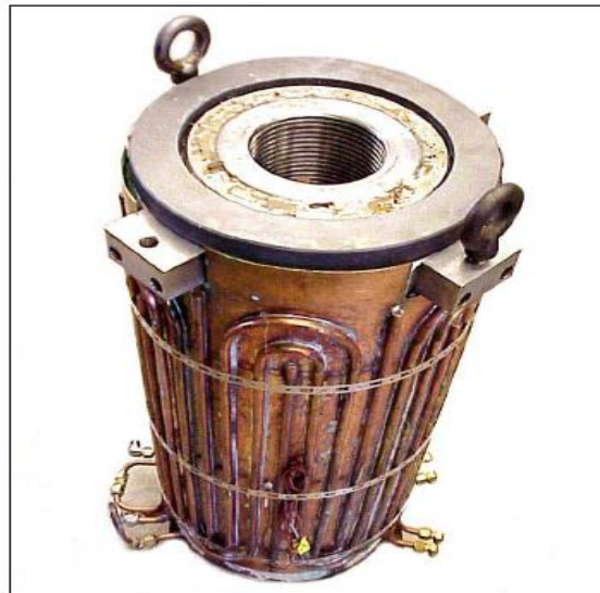
Figure 3.8 High Pressure Low Temperature Pressure Vessel with external cooling system to be used for axisymmetric compression and extension testing (Lee et al., 2002)
