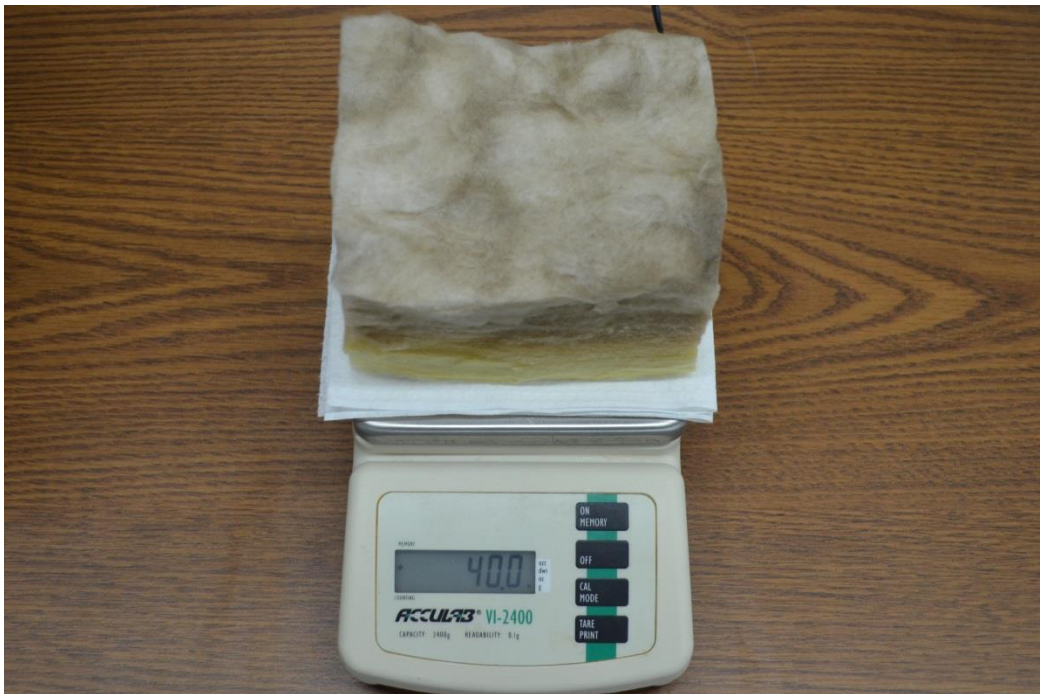
Figure 5.2 NUKON Sampling and Weighting
