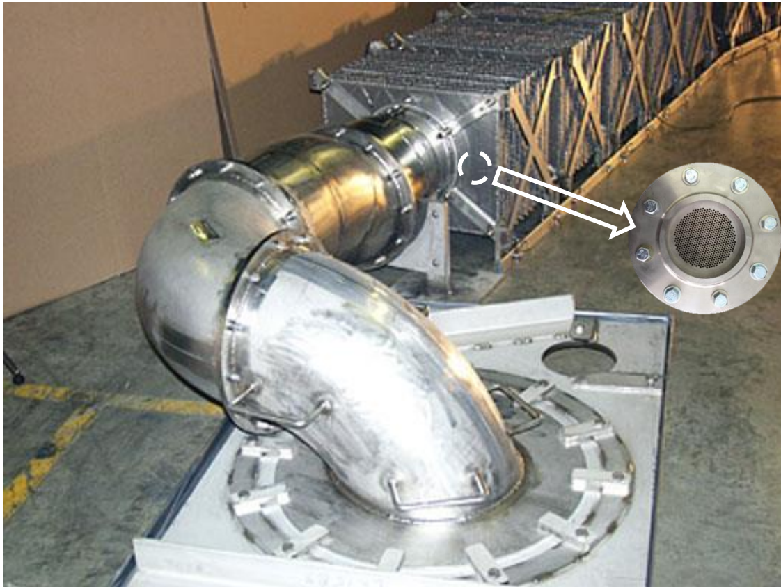
Figure 4.1 PWR Sump Strainers ( http://www.pciesg.com/sure-flow_gallery.php )
