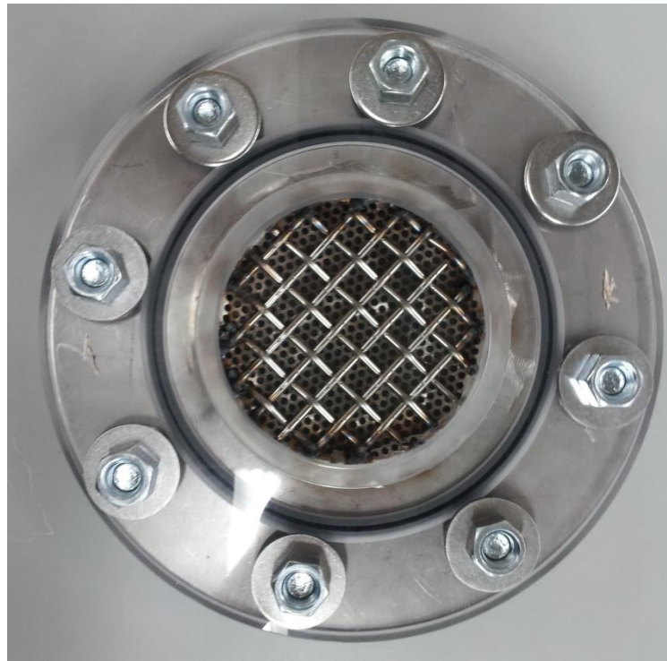
Figure 3.2 Perforated Stainless-Steel Plate with Embedded Mesh
