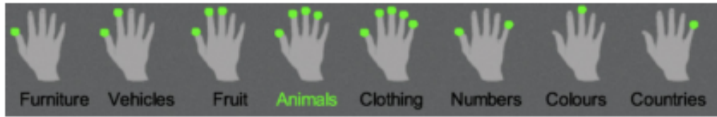
Figure 2.9: A selected set of multi-touch chords for top level item selection from Lepinski et al. [68]. When each of these are combined with a directional stroke in one of eight directions, upto 64 items can be selected.
