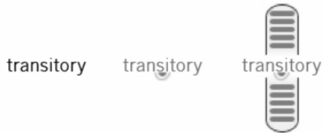
Figure 2.13: The three stages of activation of the in-context slider by Webb and Kerne [111] for parameterization of an interest value over a target.
