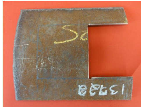
Figure 30: Material from Denting Pipe
