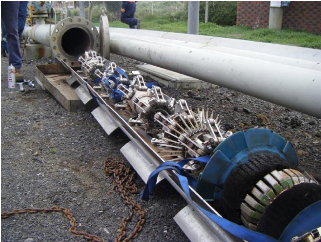
Figure 7: Pipeline Inspect Gauge (PIG) (Scott 2011)
