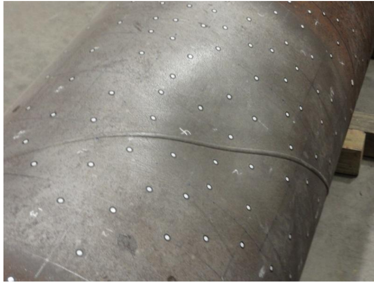
Figure 38: Smooth Dent on Spiral Weld
