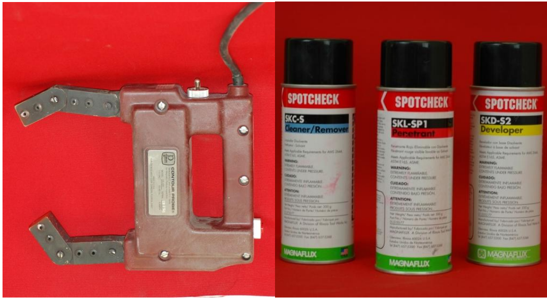
Figure 52: MPI and Dye Penetration Test
