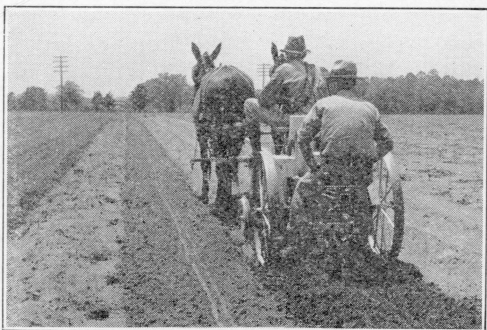
Figure 5. Rear view of special planter and fertilizer distributor, showing how top of ridge on seed bed is knocked off and how seed bed is left after all operations have been performed.
