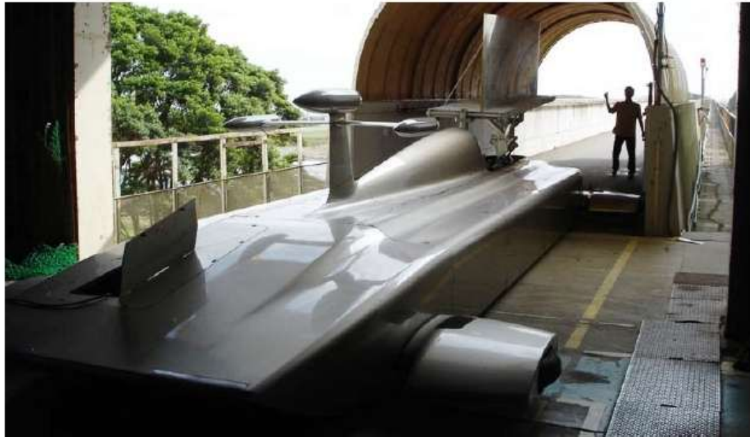
Figure 8 - Flat plate test at the Towing Wind Tunnel (Bender et al., 2007)
