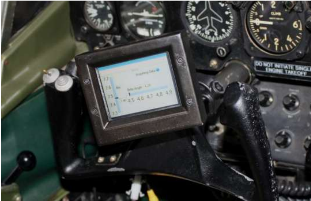
Figure 28 - Yoke-mounted pilot display
