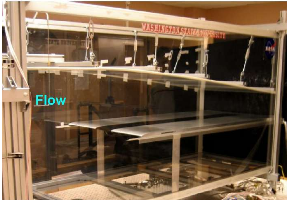
Figure 6 - Contractionless Boundary Layer Wind Tunnel (Bender et al., 2005)
