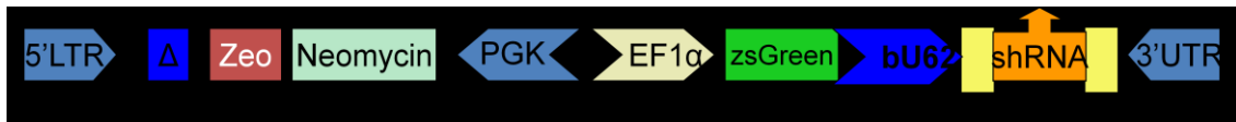
Fig. 5. Nef-GT bPol III mir-30 Based shRNA Lentiviral Expression Vectors. Transgene has dual opposing Pol II promoters. Elongation Factor 1 \alpha promoter is responsible for driving the fluorescent marker zsGreen. The Phosphoglycerate Kinase (PGK) promoter is responsible for the expression of the antibiotic resistance, G418 selection gene, and zeocin resistance as well. In addition each vector has a bovine Pol III promoter sequence directly upstream of the mir30 shRNA expression region, making unique bPol III shRNA expression cassettes. A. Is a representation of Nef-GT b7sk, B. Nef-GT bH1, C. Nef-GT bU6-2.
