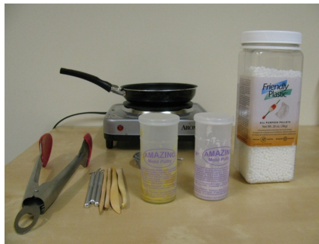
Figure 21: Tools and materials used for making physical models out of plastic in Plastic Building and Plastic Constrained Sketching conditions.
