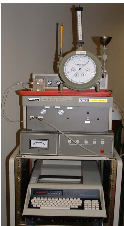
Fig. 3.7 – Carle SX gas chromatograph with a Spectra Physics SP4100 integrator.
