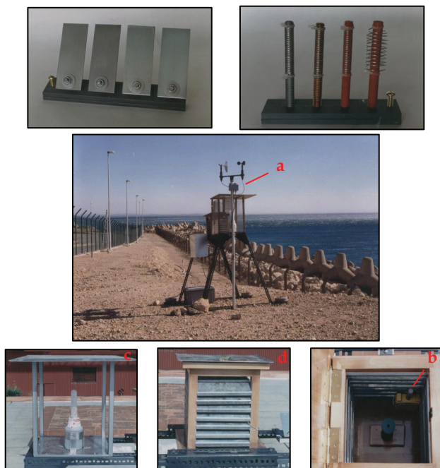
Fig. 3. View of a corrosion station (and corrosion samples) equipped with devices for recording meteorological (wind speed and direction (a), temperature and relative humidity (b)) and pollution (salinity (c) and SO 2 (d)) parameters
