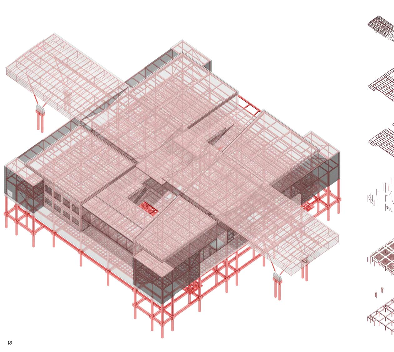
Steel supports two roofs, with a main roof covering the main masses and a secondary roof element that crosses over the top of the building, perpendicular to the atrium. This secondary roof is much lighter, constructed of tube steel trusses and stiffened with steel cables.
