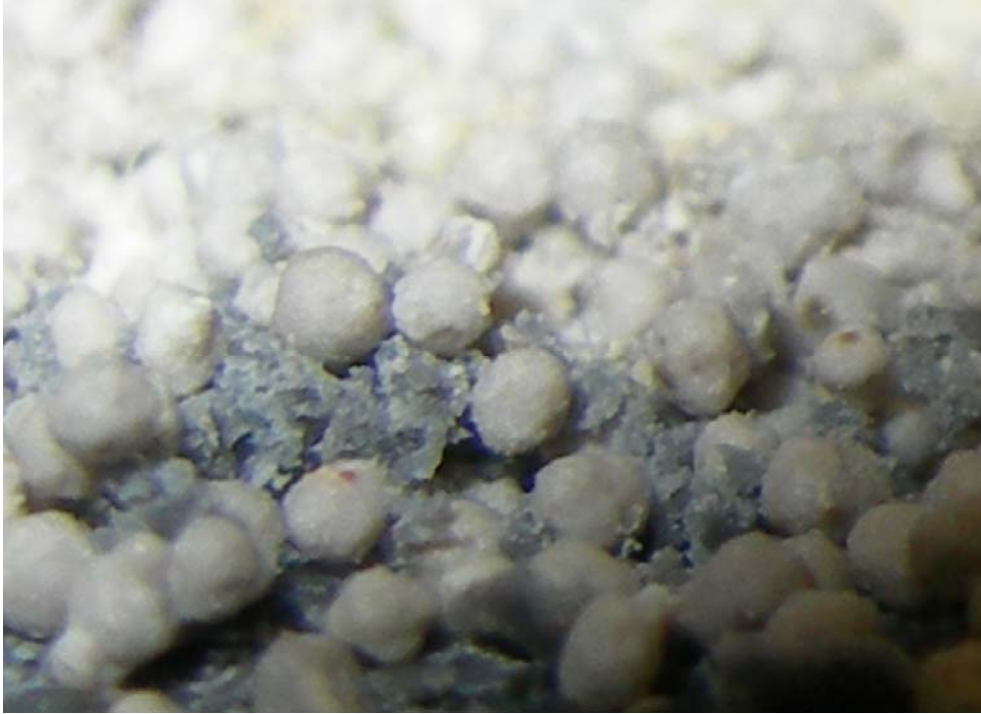
Figure D.3—Proppant with polymer residue from one laboratory test (from Chen et al at Texas A&M University 2007)
