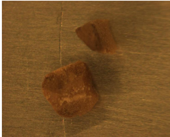
Figure 36(a). OM image of uncoated walnut shells at 175 °C
