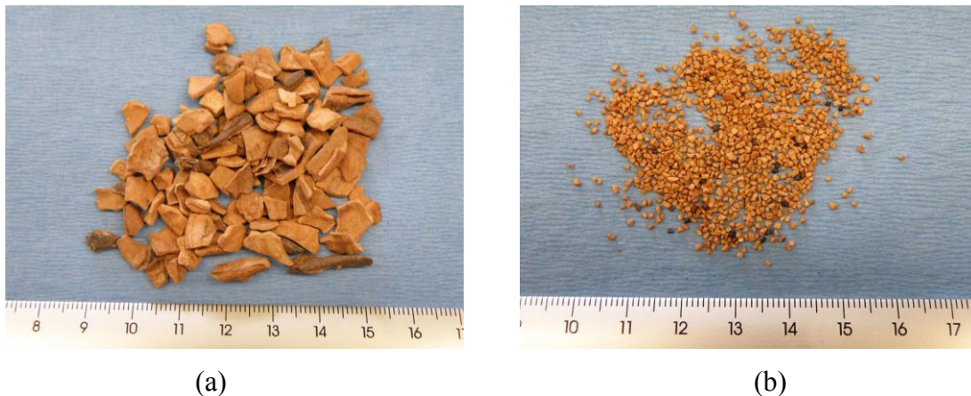
Figure 3. (a)Image of walnut shell flakes and (b) Image of coated walnut shell proppants
