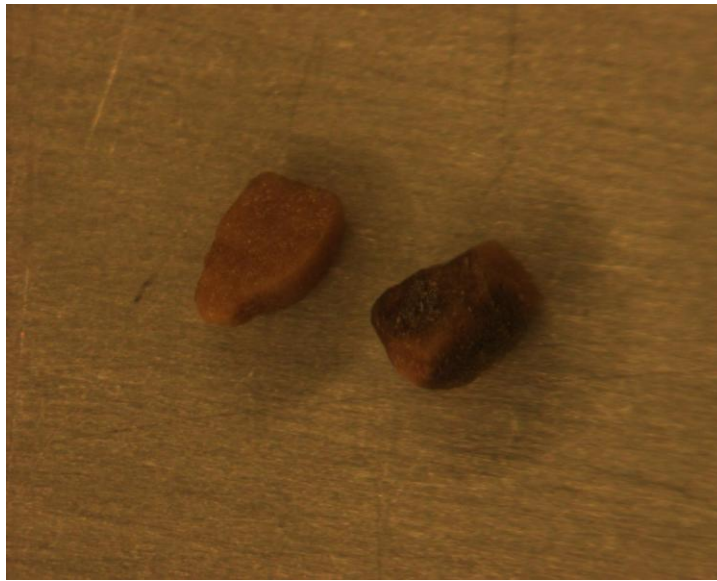
Figure 37(a). OM image of coated walnut shells at 175 °C
