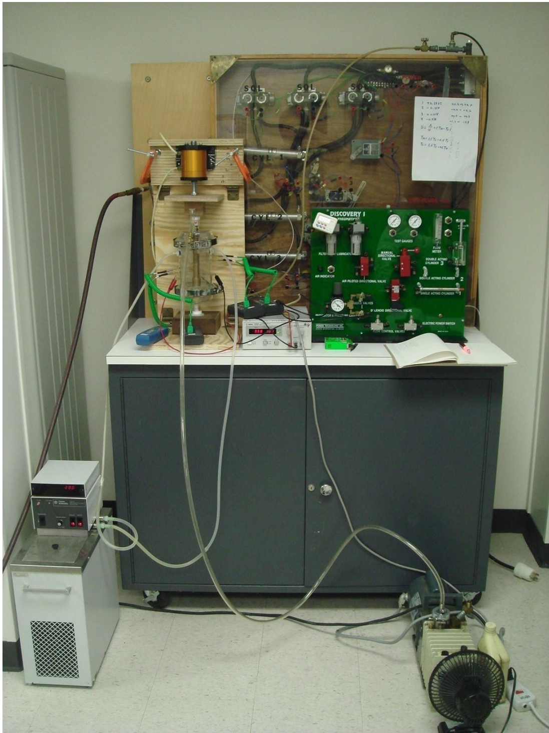
Figure 13 Image of the experimental setup used to determine thermal properties of TIMs.
