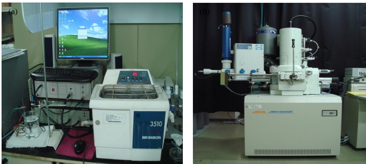
Figure 6 Images of instruments used for the fabrication and characterization of copper nanowires. (a) Ultrasonic cleaner (Branson 3510), (b) Field emission scanning electron microscope (FE-SEM) (JEOL JSM-6500F).
