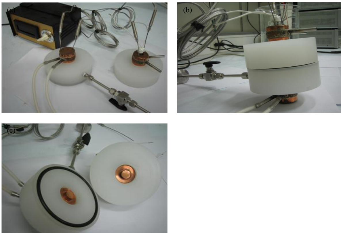
Figure 57 Images of the revised experimental fixture. (a) Thermocouple probes fixed inside copper meter bars, (b) the alignment of copper meter bars, (c) copper meter bars insulated in Polyethylene experimental fixture.
