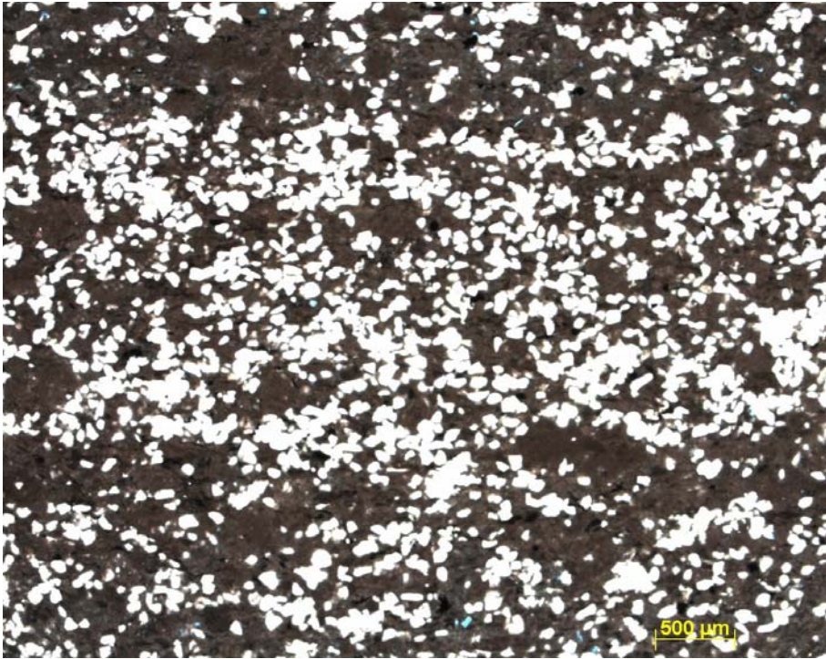
Figure D.16: Siliciclastic silty wackestone from M3, 5337'. Possible marker bed below Sunflower pay.
