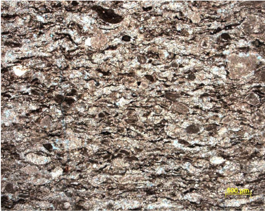
Figure D.12: Packstone facies with unidentifiable peloidal grains; displays H1-Br porosity after mechanical grain compaction. Sample M3, 5305.
