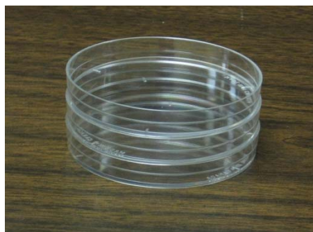
Figure IV-2 – The three-chamber phantom used for spectroscopy. Contains three phosphorus compounds with different chemical shifts that mimic biological content.
