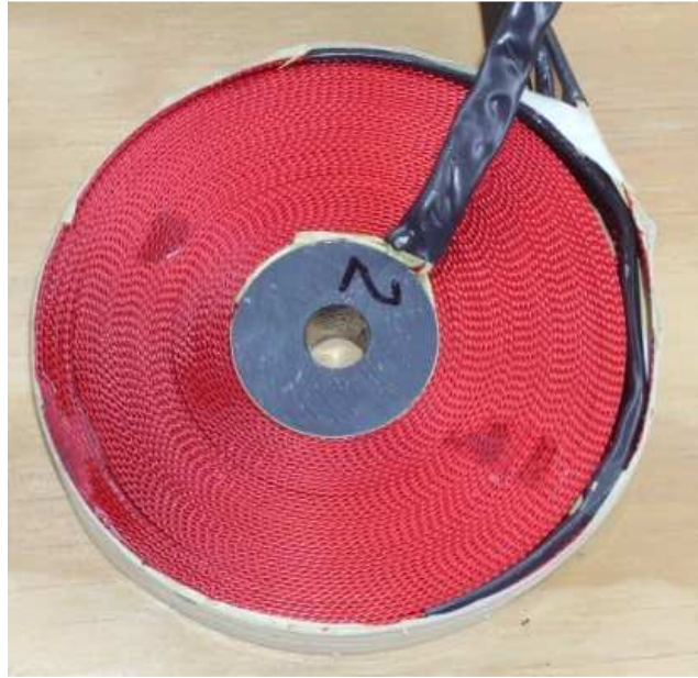
Fig. 20. 100 \mu\text{H} link inductor for 15 kW prototype
