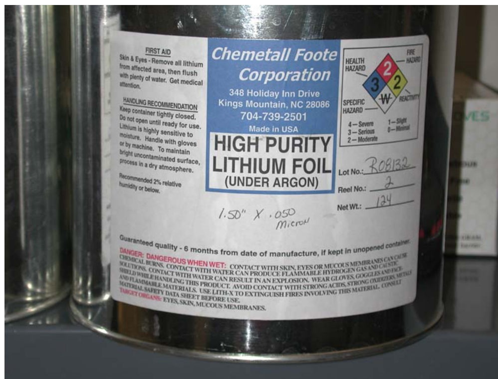
Fig. 41. Ninety-five percent enriched lithium-6 metallization material.
