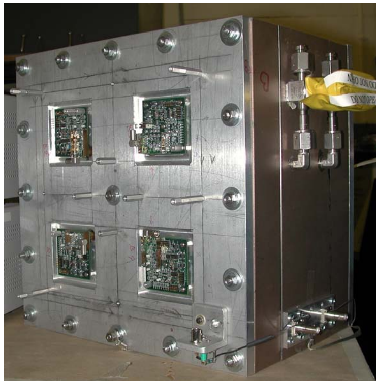
Fig. 44. Fully assembled detector array with detector electronics.
