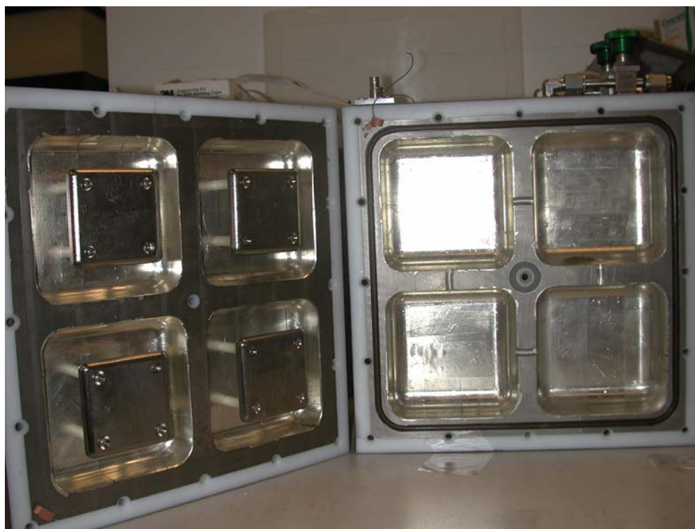
Fig. 42. Lithium metallization is applied on the interior surface.
