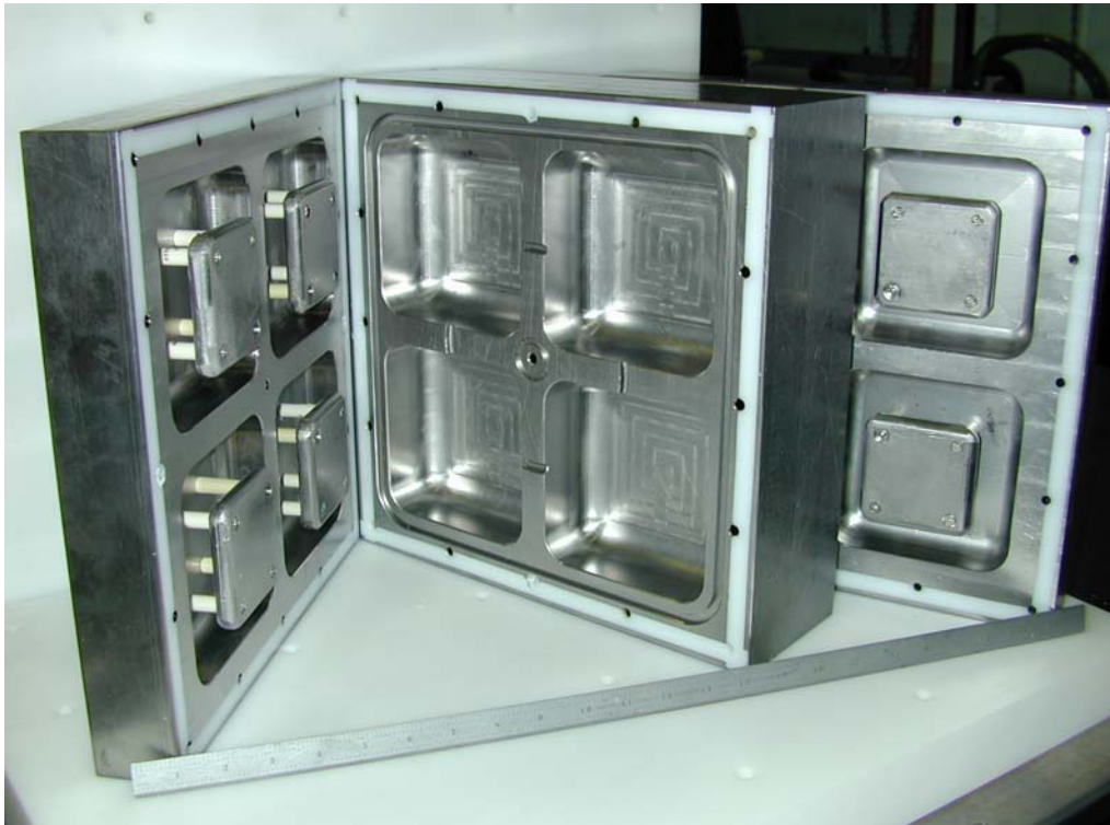
Fig. 33. Polyethylene body with 8-micro thick nickel and stainless steel metallization.
