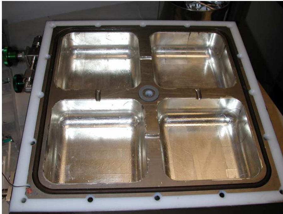
Fig. 43. Close-up of the lithium metallization.
