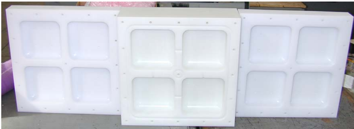
Fig. 32. Machined, bare polyethylene body; 2 lids and 1 middle piece (center).
