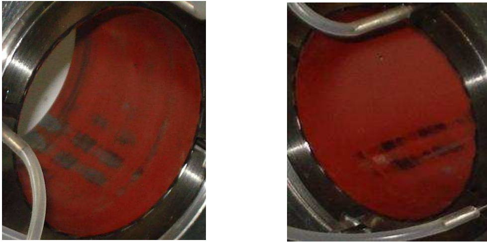
Figure 48: Top foil wear after Test 6; 35,000 RPM with supply pressure of 80 psi and 14 SCFH air flow
