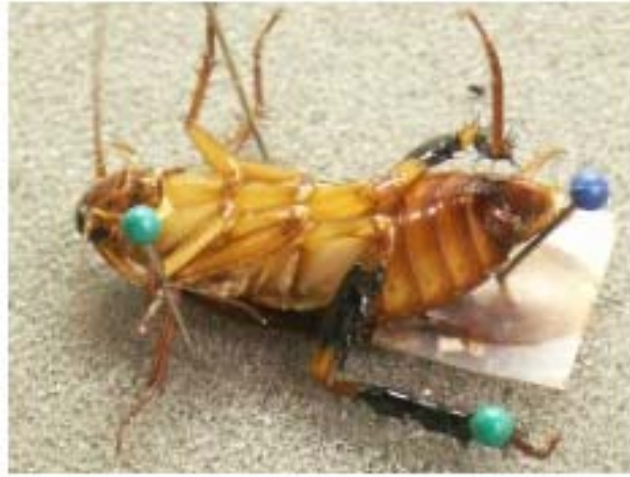
Figure 20: Latex paint around femur and tibia provide a good surface to bond or tape the sensors. Latex paint shrinks slightly while drying making bonding less of an issue.
