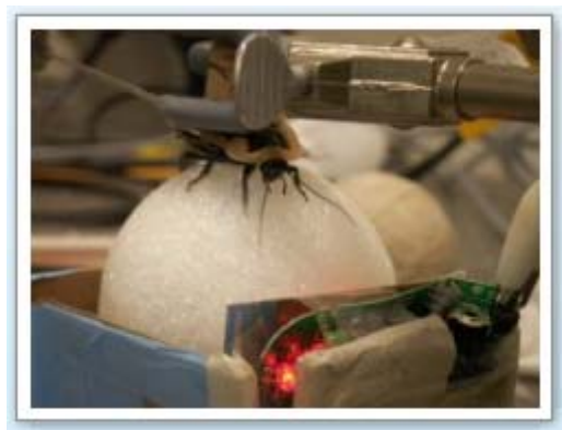
Figure 22: Roach tracking device with roach held fixed with a beaker holder. As the roach tries to walk, it moves the ball which is tracked by the optical mouse. While Blaberus was capable of moving the ball with ease, Periplaneta had more difficulty and tired quickly.
