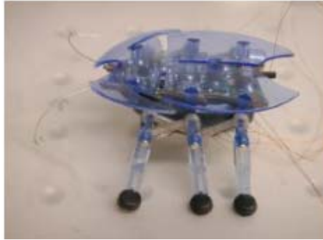
Figure 29: Hexapod robot simulates tripod walking pattern of the cockroach for sensor validation.
