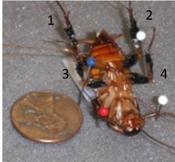
Figure 34: Roach with four sensors installed, one on each of the mesothoracic and metathoracic legs at the femur-tibia joints.
