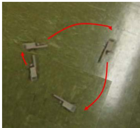
Figure 41: Roach with right turning device makes a clockwise circle during walking.
