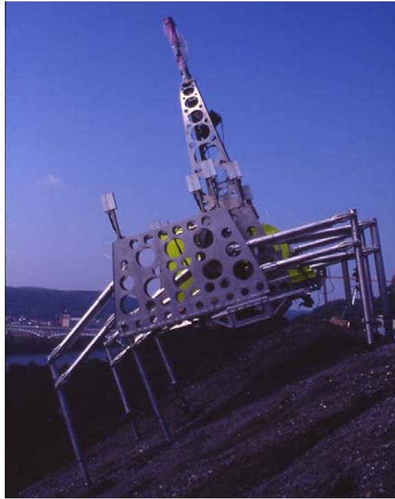
Figure 2: Dante II on its voyage into a volcano. Although guided by human operators, Dante proved its ability at navigating through uneven terrain. [10]
